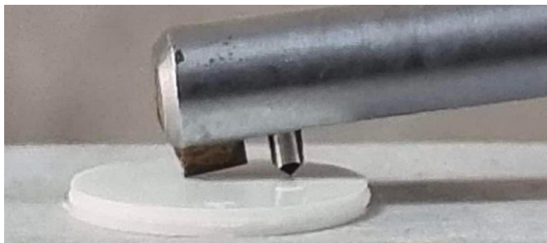
Figure 2: Disc-shaped specimen put in profilometer for roughness test
