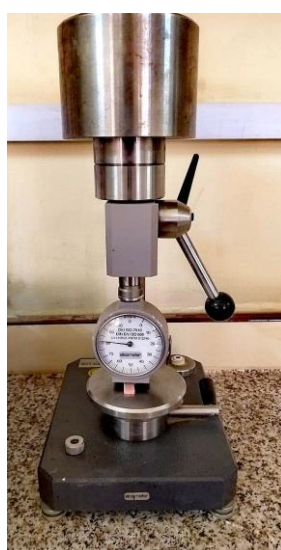
Fig. (4) Dorometer 3120 hardness test device, type (Shore D)
