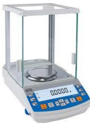
Fig. (2) Sensitive balance high accuracy.
