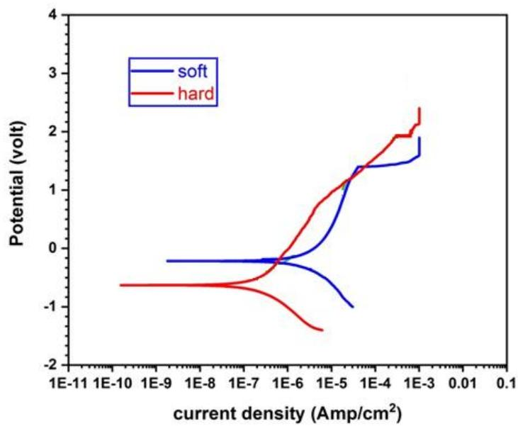
Fig. (7) Polarization curve for Co- Cr samples
