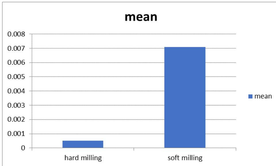
Fig. (8) Bar chart of the corrosion test (mmpy) for two hard milling and soft milling groups.
