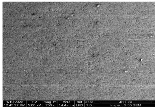
Fig. (4) SEM results for a soft milling sample before heat treatment.
