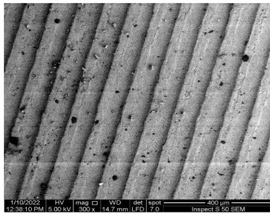
Fig. (3) SEM results for a hard milling sample before heat treatment.
