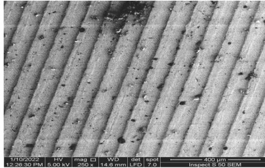
Fig. (5) SEM image of the sample surface during hard milling after heat treatment.
