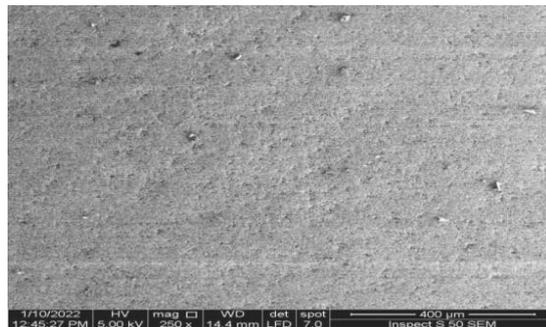
Fig. (6) SEM image of the surface of the soft milled sample after heat treatment
