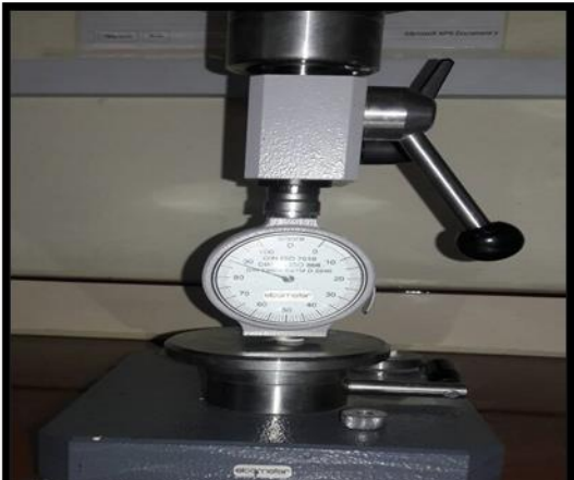
Fig. (2): Surface hardness (Shore D) testing unit
