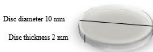
Figure (1): Shape and dimensions disc of surface roughness sample of all tested materials
