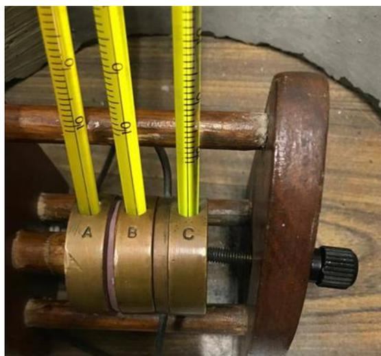
**Figure 2:** Thermal conductivity apparatus ( Lee disc).
