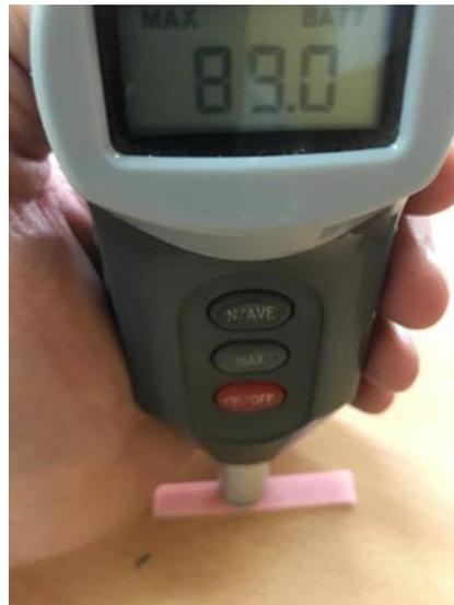
Figure 4: Specimen testing with hardness device.
