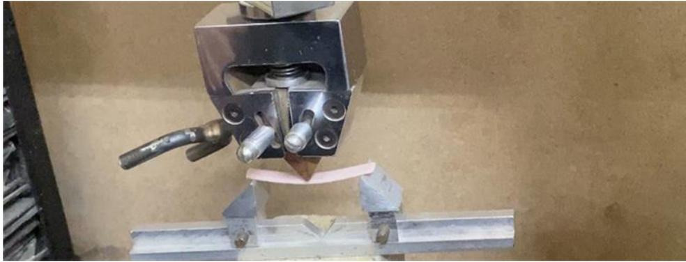
Figure 3: Specimen bending before fracture.
